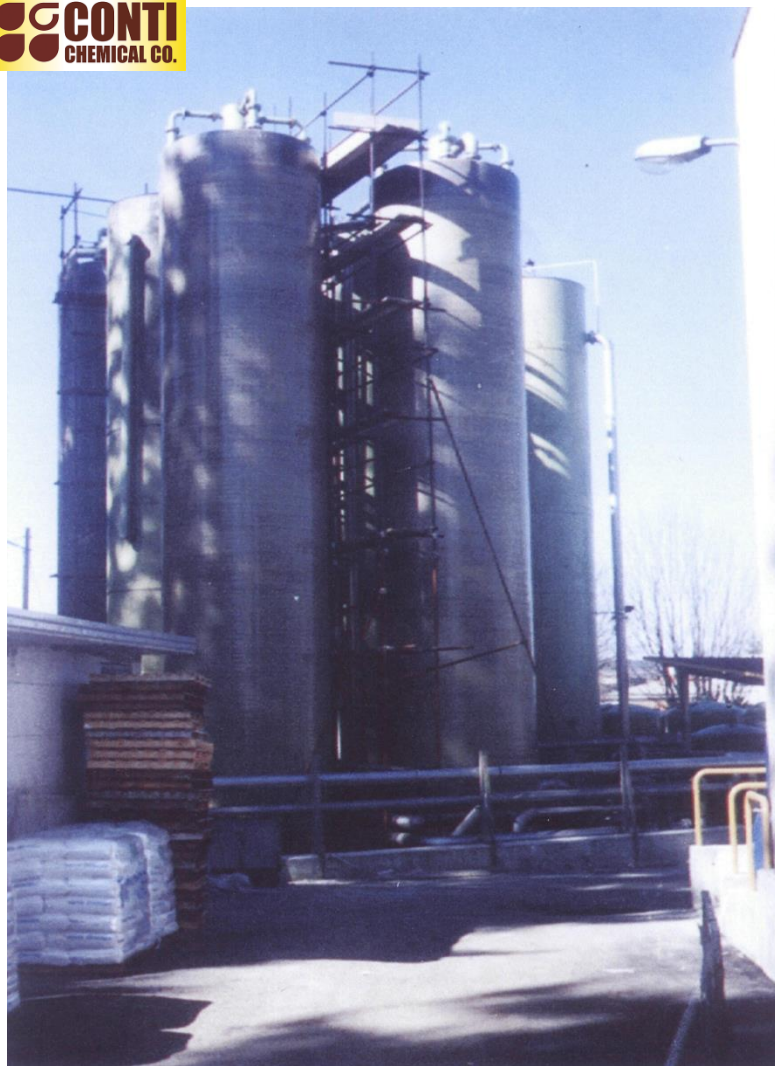
Local WWTP of silk dyeing factory Timesta. Capacity 2000 m 3 per day. 1998, Como, Italy
